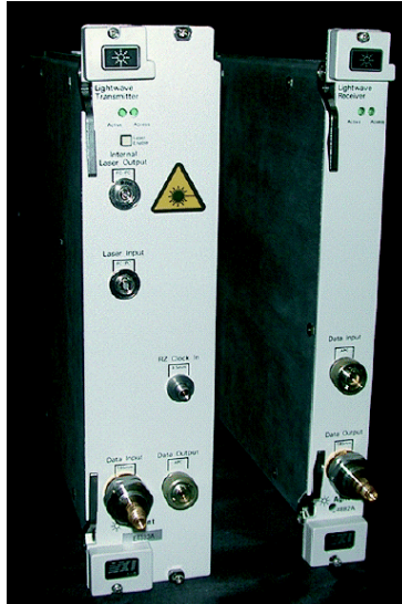
Figure 75 E4883A Transmitter (E/O Converter) and E4882A Receiver (O/E Converter)
