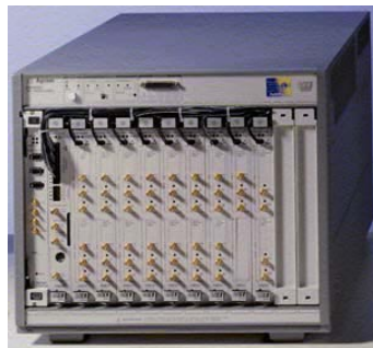
Figure 2 E4803A Mainframe with Modules
